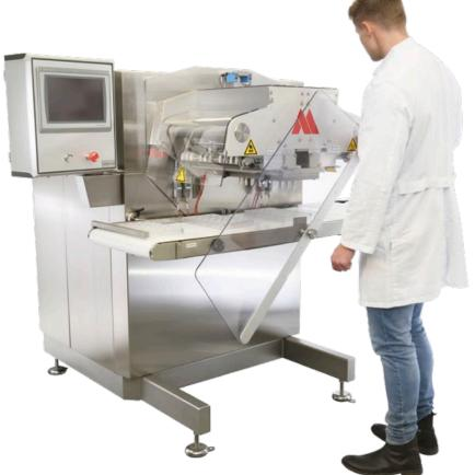
The Nilshot works with many types of moulds, and the flexibility of the pistons allows full control of the production. The turnable safety screen insures safety for the operator and allows for easy access, when it is in open position.
